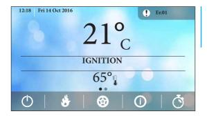
Blocking or non-blocking error is highlighted with a  $\P$  and the related error code. When pressed the error window opens
