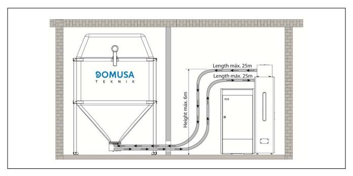
**IMPORTANT:** At each end of the pellet suction and air return hose, the copper cables must be connected to the earth connection terminals provided on the **Silo** for this purpose.
