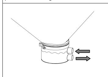
Connect the pneumatic suction system hoses as shown in the figure and fix them in place with the clamps supplied with the Silo.
