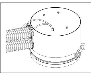
Both the suction pot and the suction system hoses must be earthed. The underside of the suction pot is designed for an earth connection terminal to be bolted to it.
