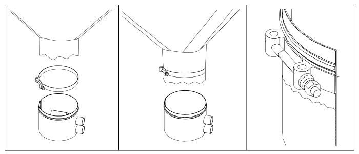
Place the canvas around the outside of the suction pot and fix the clamp to the upper part of the pot, as shown in the figure.
