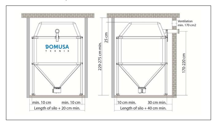
Example of installation of the Textile Silo in the same room of the boiler room:
