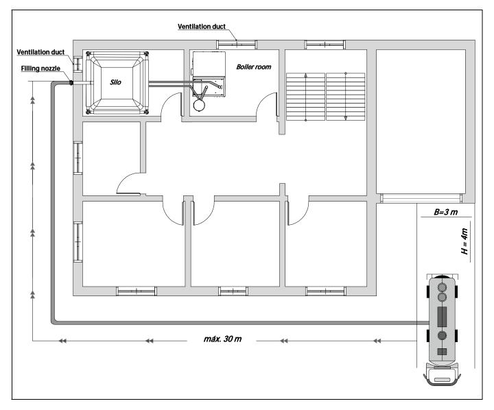
**IMPORTANT:** For safe Silo filling it is essential for the filling nozzle and supply hose to be earthed during the filling process.
